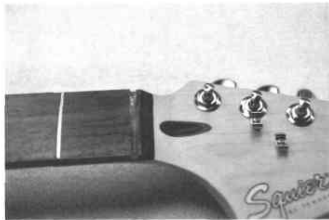
The Fender Squier, after removal of the original nut.
