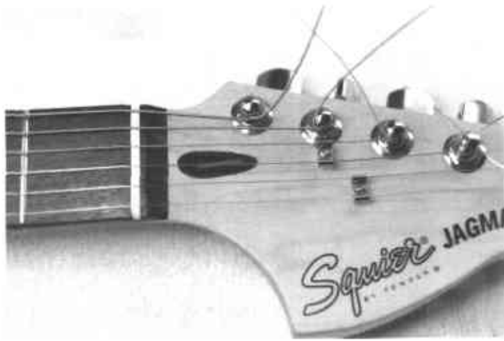
The Fender Squier prior to removal of the original non-compensated nut
